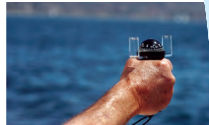
(Top) The Weems & Plath hockey puck style compass allows for easier and more accurate sighting on the move than the pistol style compass pictured below it.
